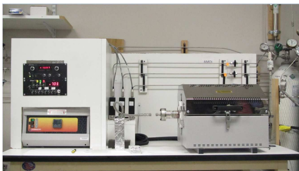
Figure 4.5: Optical image of the CVD system to be used for graphene synthesis in our lab.
